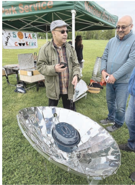
Parabolic cookers adjust to follow the path of the sun to maximize heat for cooking.
